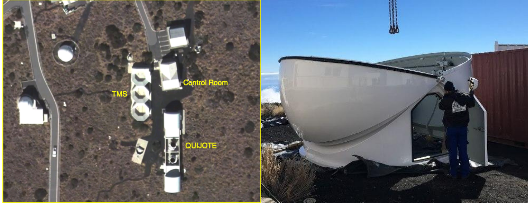
Figure 3. Left: Location of the former VSA platform at the Teide Observatory. The TMS dome will be installed in the central enclosure (marked as TMS). Right: Fiberglass AllSky dome installed for the GroundBird experiment at the Teide Observatory. The TMS dome, to be installed in the second enclosure, is similar to this one.
